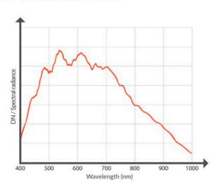
The Specim FX10+ is a high-speed line-scan hyperspectral camera optimized for applications requiring fast imaging. Its high resolution ensures accurate and detailed imaging at a rapid pace. Specim FX10+ operates in the visible and nearinfrared (VNIR) region from 400 to 1000 nm.
